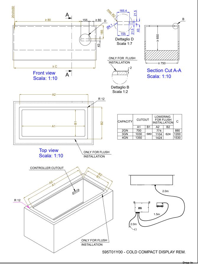
Drop-in Drop-in remote refrigerated well with refrigerated display, compact (4 GN container capacity) The company reserves the right to make modifications to the products without prior notice. All information correct at time of printing.
